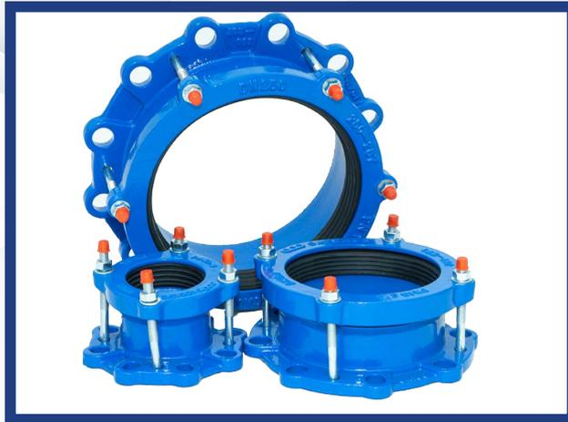
For use in joining pipes within a range OD's to flanges. Cast in ductile iron Grade 420/12 to BS2789:1985. PE coated to:
