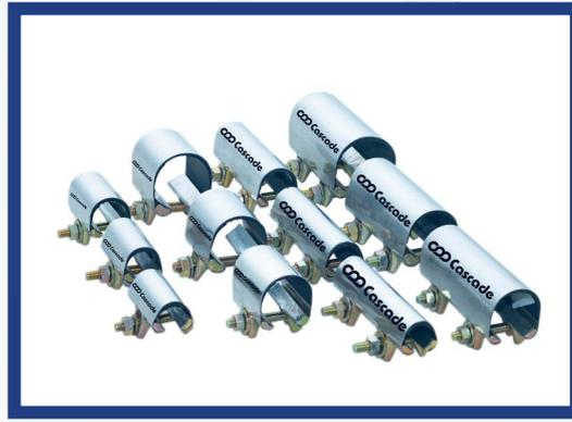
Cascade half clamps are used for repairing pin-hole breaks in smaller diameter pipes. They provide a quick, easy, and cost-effective solution for this type of break. Cascade half clamps are available in sizes to suit galvanised pipe from 1/2" (15mm) through to 2" (50mm). Standard lengths are 75mm and 150mm.
