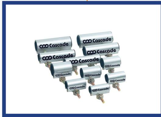
Cascade junior couplings provide a quick, easy, and cost-effective solution for repairing larger breaks in smaller diameter pipes. It provides a full circumference seal around the pipe. Available in sizes to suit galvanised and copper pipe from 1/2" (15mm) to 1 1/4" (32mm).
