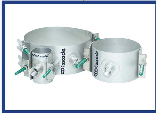
The flexible stainless-steel band allows for easy fitting while wrapping fully around the pipe, providing support and stability – eliminating the “crushing effect” of more rigid products. The band is recessed to correctly position the “O” ring gasket and provide maximum sealing. Recommended for PVC pipe and manufactured to suit sizes up to 14” Cascade service saddles can be fitted with 1/2” through to 2” diameter sockets.
