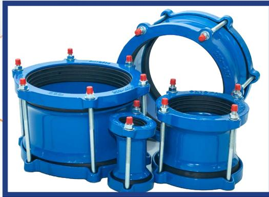
Wide range couplings suitable for joining pipes with the same nominal diameter – which have the same or different OD's. Cast in ductile iron Grade 420/12 to BS 2789:1985.
