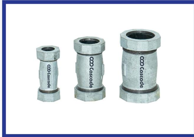
Precision cast in malleable cast iron to BS6681 B32-10 enabling easy fitting. The prominent “centre-hex” affords a secure grip of the fitting to be made, allowing the end caps to be tightened with ease. The couplings are galvanised to provide protection against corrosion. NBR rubber to ISO 4658-1990, BS2751-1990.
